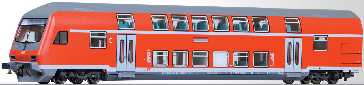
Doppelstock-Steuernwagen 2. Klasse DBbzf 761 der DB AG 2nd class double-deck driving cab coach DBbzf 761 of the DB AG
